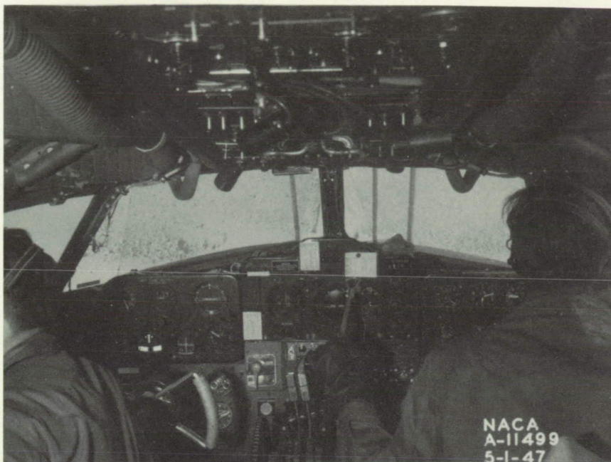
Figure 21.- Typical ice accretion on V-type windshield without any heat supplied.
