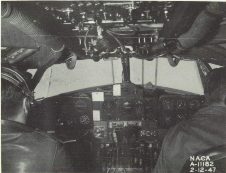
Figure 20.- V-type windshield of C-46 airplane during flight in icing conditions showing unsuccessful ice-removal operation of external discharge jets over pilot's panel, with heat supply of 18,000 Btu per hour.
