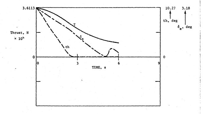
Figure 4b. Flare response: thrust, throttle, and elevator; wind profile b.
