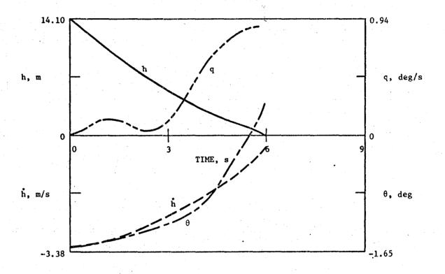
Figure 10a. Flare response: altitude, sink rate, pitch, and pitch rate; wind profile H.
