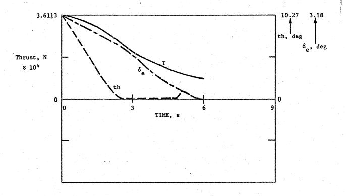
Figure 10b. Flare response: thrust, throttle, and elevator; wind profile H.
