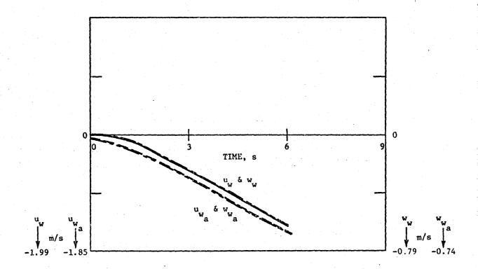
Figure 6c. Flare response: wind velocity components at the wing; wind profile D.
