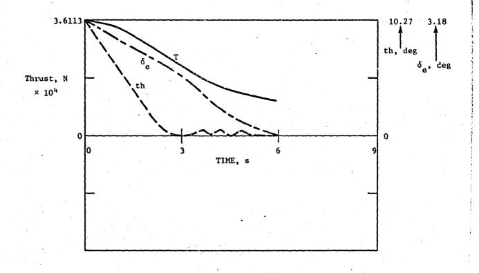
Figure 9b. Flare response: thrust, throttle, and elevator; wind profile G.
