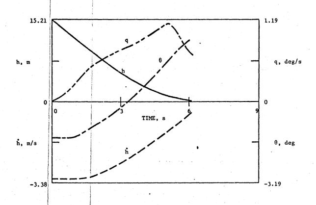
Figure 5a. Flare response: altitude, sink rate, pitch, and pitch rate; wind profile C.
