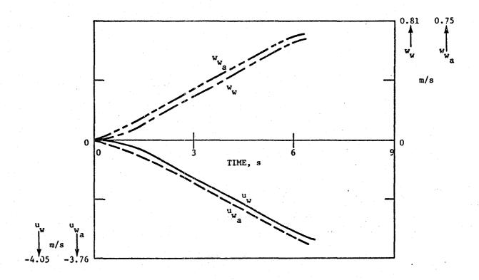
Figure 5c. Flare response: wind velocity components at the wing; wind profile C.
