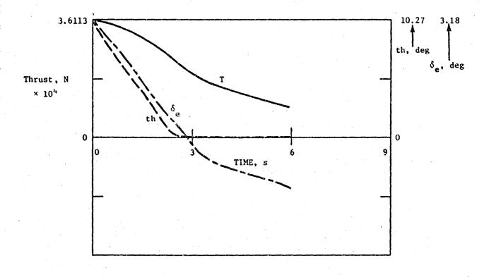
Figure 8b. Flare response: thrust, throttle, and elevator; wind profile F.
