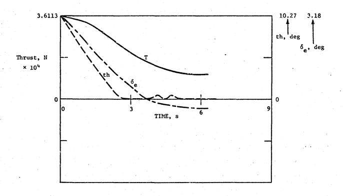
Figure 7b. Flare response: thrust, throttle, and elevator; wind profile E.
