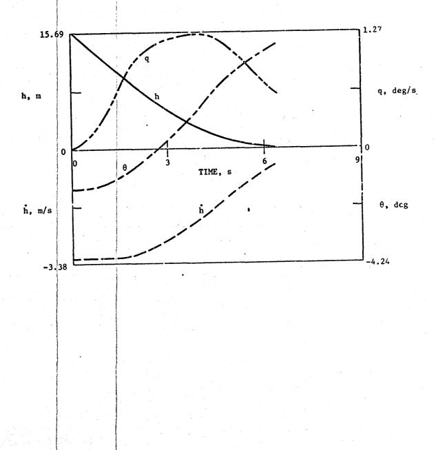
Figure 7a. Flare response: altitude, sink rate, pitch, and pitch rate; wind profile E.
