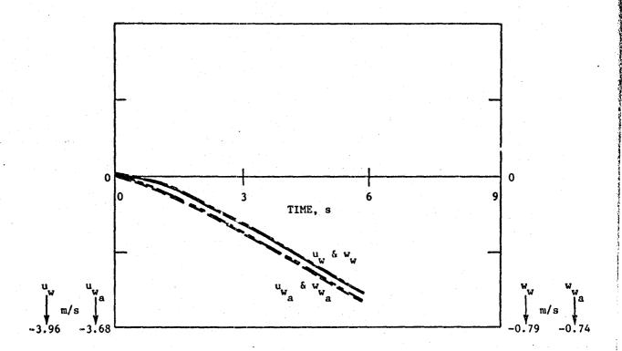
Figure 4c. Flare response: wind velocity components at the wing; wind profile B.
