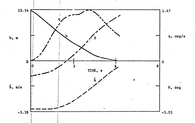
Figure 3a. Flare response: altitude, sink rate, pitch, and pitch rate; wind profile A.
