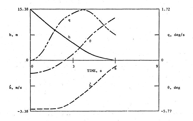
Figure 8a. Flare response: altitude, sink rate, pitch, and pitch rate; wind profile F.
