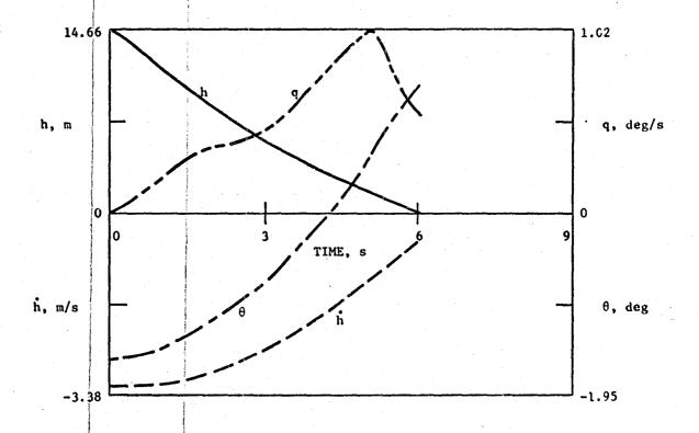
Figure 4a. Flare response: altitude, sink rate, pitch and pitch rate; wind profile B.
