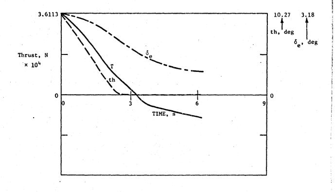
Figure 3b. Flare response: thrust, throttle, and elevator; wind profile A.
