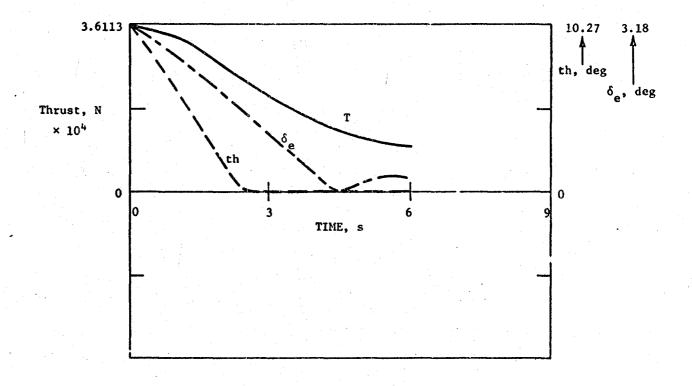
Figure 6b. Flare response: thrust, throttle, and elevator; wind profile D.
