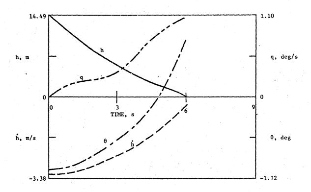
Figure 9a. Flare response: altitude, sink rate, pitch, and pitch rate; wind profile G.
