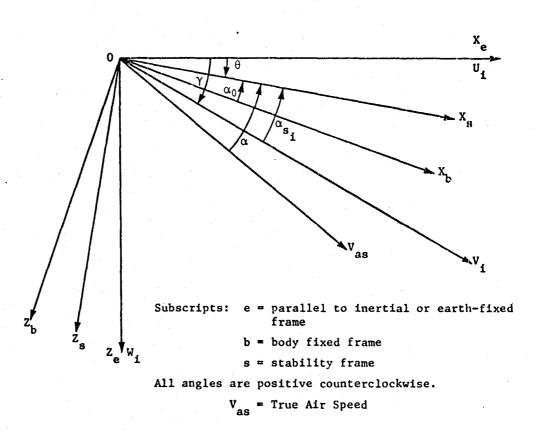
Figure 1. Coordinate frame and flight geometry.
