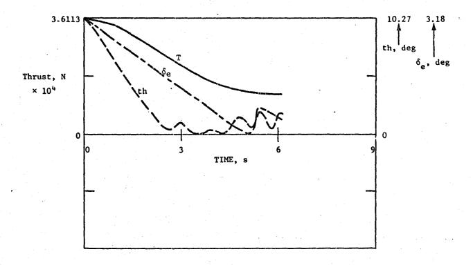
Figure 5b. Flare response: thrust, throttle, and elevator; wind profile C.
