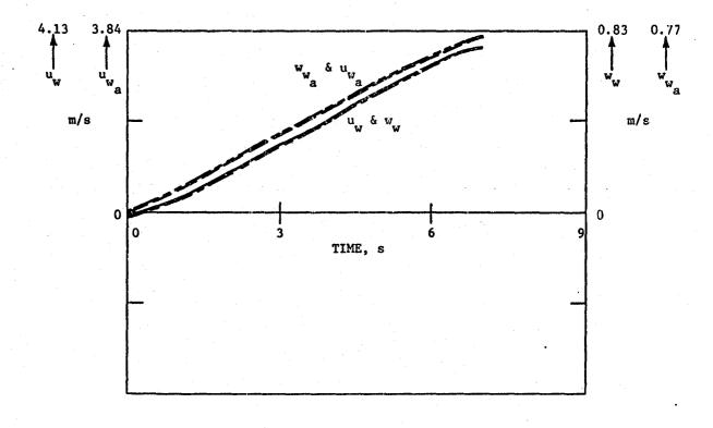
Figure 3c. Flare response: wind velocity components at the wing; wind profile A.
