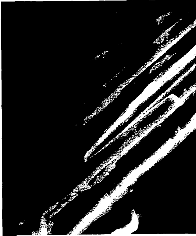
(a) Specimen No. 15, 3 \times 10^9 Rads Dose at 120^\circ\text{C} , Tested In Vacuo
