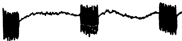
Fig. 4. Optically detected 2.5 MHz gated pulse signal.
