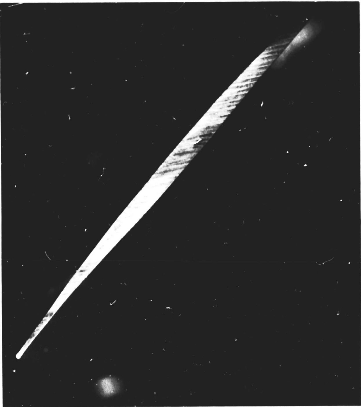
Figure 8 Compressor Blade Tip After Rubbing. The blades were in good condition after the intentional rub-in of the compressor.
