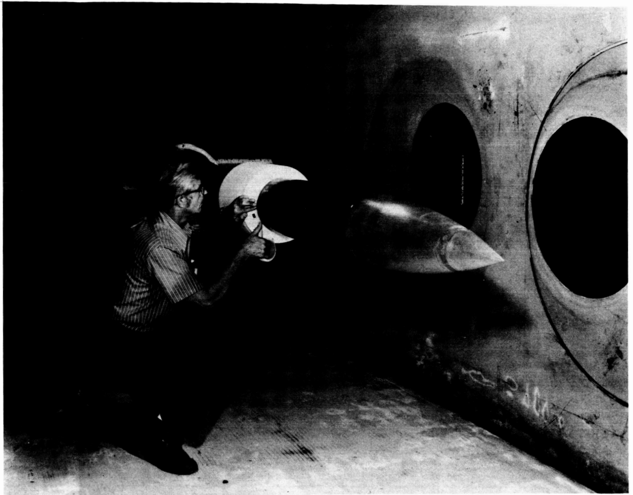
Figure 2.— Ogive-cylinder model with \theta = 45^\circ cone frustum and axisymmetric ring.
