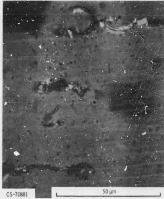
Figure 7. - Abrasive wear debris (from ref. 9).
