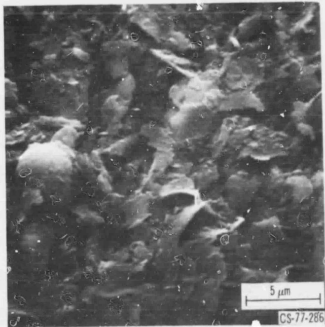
Figure 4. - Normal rubbing wear particles (from ref. 8).
