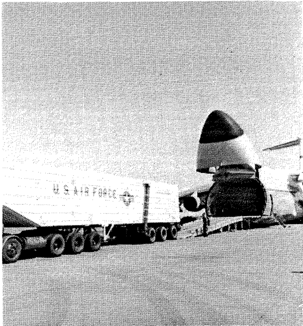
Figure 41. C-5 Aircraft Being Loaded through Nose-Visor Door on Forward Fuselage
