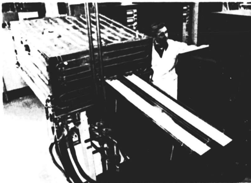
Figure 18. SCIM-II exterior showing two side-by-side substrates entering the coater.
