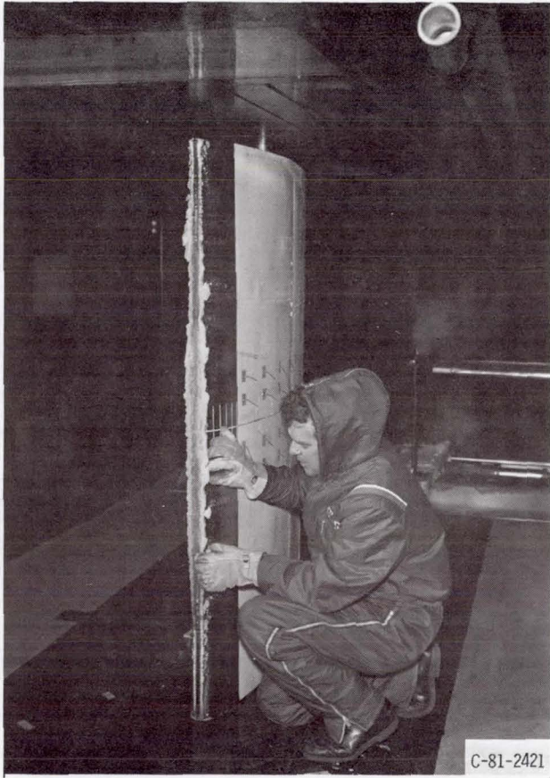
Figure 3. - NACA 63 2 -A415 wing section mounted in Icing Research Tunnel.
