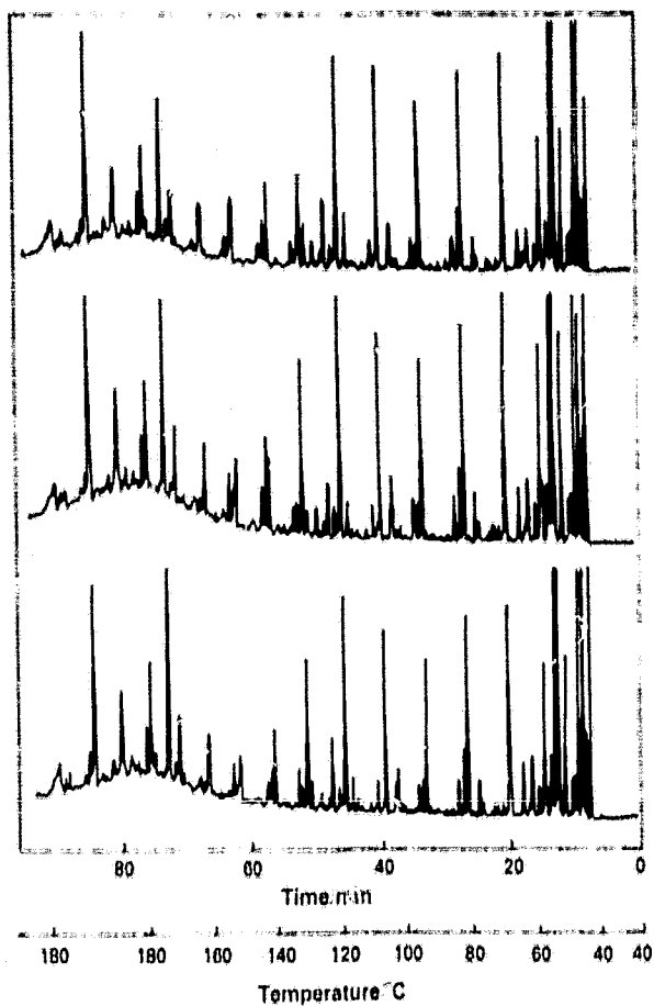
Figure 4. Repeatability of the transelevator sampling technique in the solvent elution mode for three 50 \mu l samples of a pooled normal serum. The three replicate separations were performed on a 106 m x 0.25 mm i.d. glass capillary column coated with Silar 10C. The column was programmed with an initial isothermal period at 40°C for 6 min, then programmed at 2°C min -1 to 180°C and held at this temperature for 30 min. Helium carrier gas flow rate, 1.5 ml min -1 .
