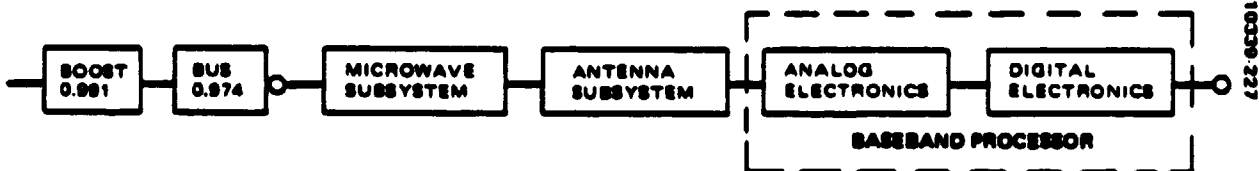
FIGURE 4.3-1. 30/20 GHZ PAYLOAD RELIABILITY BLOCK DIAGRAM
