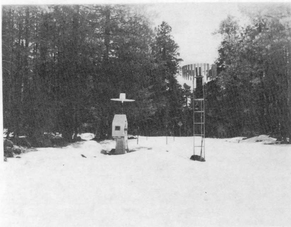
Figure 32. Snow-monitoring site at Baker Butte equipped with a Landsat data-collection platform.
