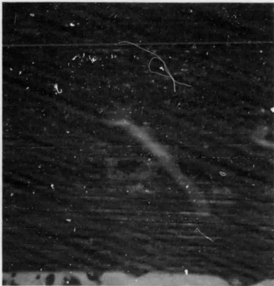
Figure 7. Top plates and separators removed to reveal more "bridging" in cell No. 3.
