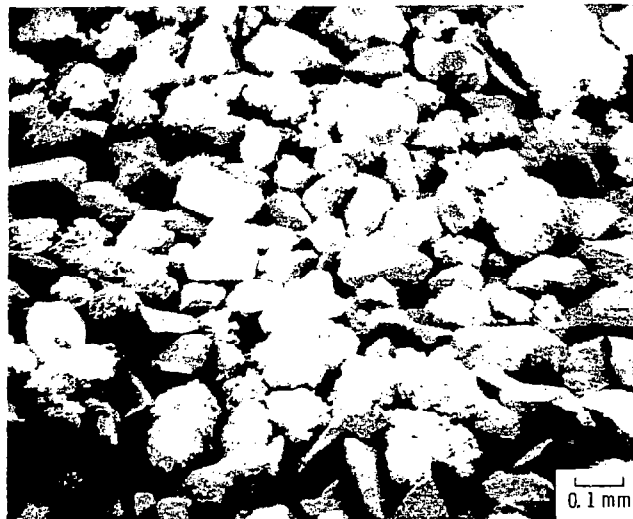
(c) Batch 3, for coating 3 powder, made with -5 \mu\text{m} and -150, +325 mesh \text{CaF}_2 powders and 6.25 wt% \text{AlPO}_4 binder.
