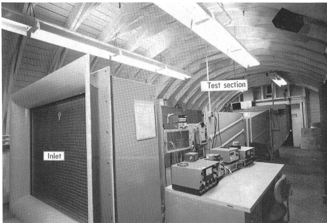
Figure 3.- Low-velocity calibration wind tunnel at the Langley Research Center.
