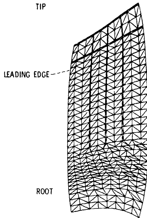
Figure 1 - Nastran model of the hollow fan blade (777 elements).
