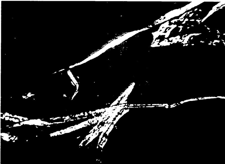
Figure 68. Contamination in Narmco Neat Resin Batch 300—Wood Fibers
