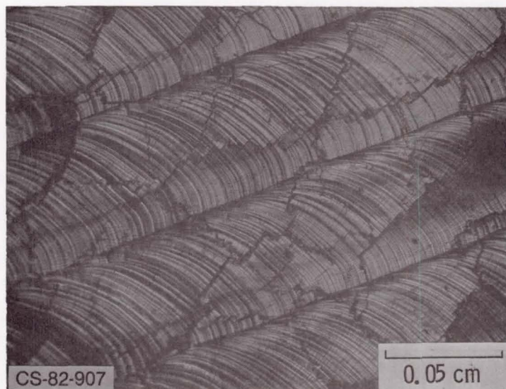
Figure 2.—Photomicrograph of a 0.020 cm thick, laser glazed ceramic coating. Power density: 35 W/mm 2 .
