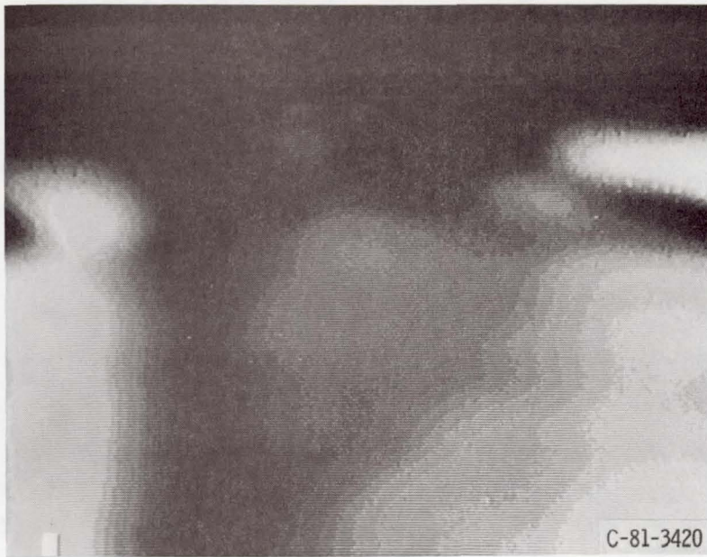
Figure 6. - Imaged damage in a 1 1/2 x 3 inch area of a broken composite specimen.
