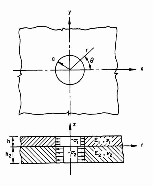
Figure 1. Geometry of the composite plate
