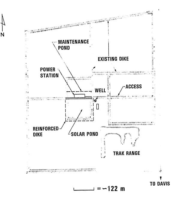
Figure 1. Site Layout for a 300  $k \ensuremath{\mathbb{W}}_e$  Solar Pond Power Plant at Davis
