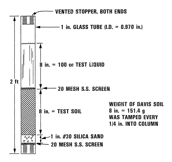
Figure A-1. Apparatus for Test of Soil Permeability
