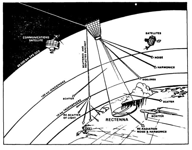
Fig. 5. SPS Electromagnetic Interference Mechanisms
