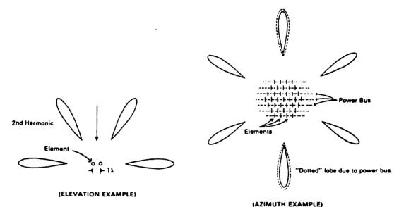
• DIRECTIONAL CHARACTERISTICS OF HARMONIC SCATTERING FROM A RECTENNA CAN BE DETERMINED BY GRATING LOBE ANALYSIS, WITH THE RECTENNA RECEIVING ELEMENTS, POWER BUS, AND OTHER RECTENNA COMPONENTS AS RADIATORS.
