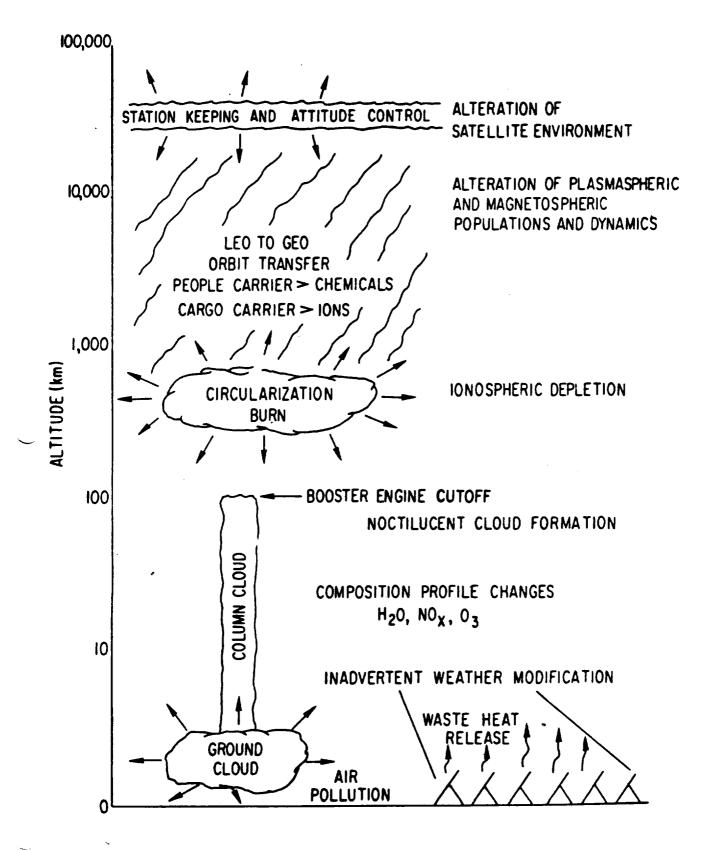
Fig. 3. Illustration of Potential SPS Atmospheric Effects
