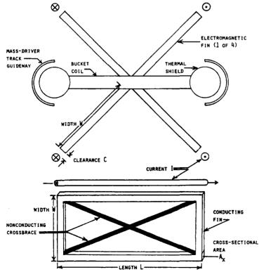
Figure 1. Block diagram of lunar mass-driver for launching of lunar materials at >10<sup>6</sup> tons/year. (Modified from Chilton et. al., AIAA Progress Series, Vol. 57, 1977, p. 40)
