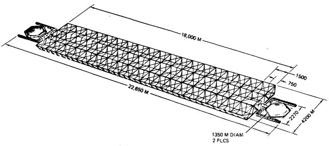
Figure 1, Solid -State End-Mounted Antenna Satellite Concept
