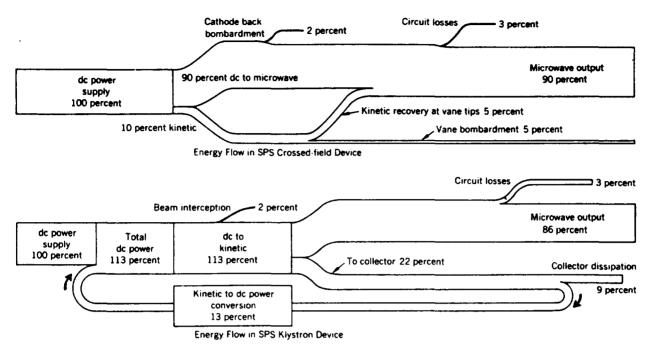
Figure 1. Comparison of DC-RF Conversion Operations for Crossed-Field (Top) and Linear-Field (Bottom) Beam Devices.
