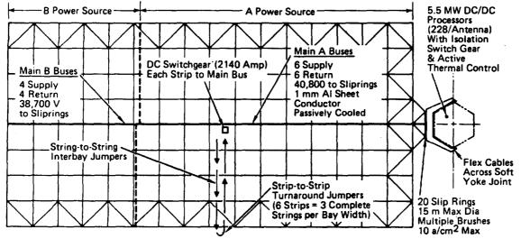
Figure 3. Multiple Bus SPS Power Distribution (Si Cells)
