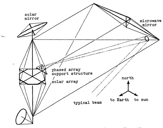
FIGURE 1: A gravity-gradient stabilized configuration, incorporating a rotating solar mirror and no rotating electrical joint. Length about 100 kilometers.
