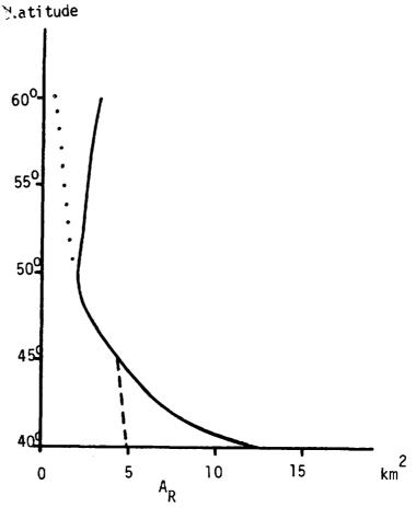
Fig. 4: Solid Curve: Rectenna area (A<sub>R</sub>) required to receive power continuously from a pair of orbits shown in Fig. 1. The curve is normalized for satellite antenna areas of  $1 \text{ km}^2$ . Dotted extension shows effect of the four additional orbits shown in Fig. 2. Dashed curve shows effect of adding the two orbits of Fig. 3.
