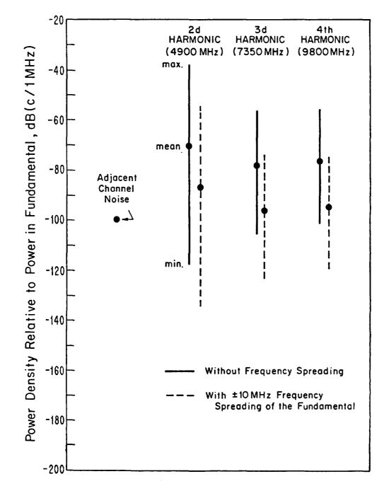
Figure 2. Estimates of interference levels in a 1 MHz bandwidth.
