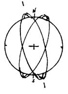
Fig. 2: Four additional orbits which could be added to those shown in Fig. 1. These circular orbits are inclined at  $\pm$  73.1° and rotated by  $\pm$  14.3° about the polar axis.
