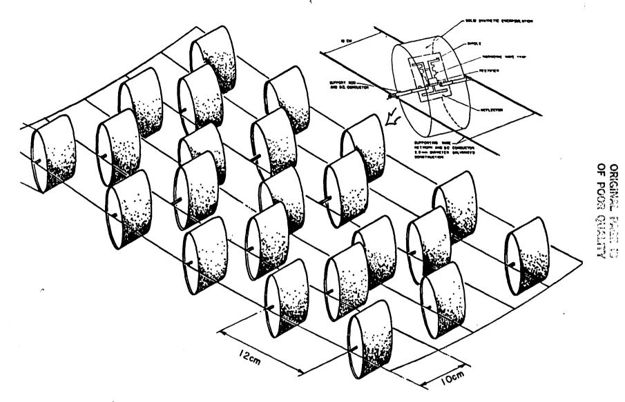
FIGURE 2. DIAGRAM SHOWING SECTION OF 100FT X 100FT NON-GROUND PLANE DIPOLE MICROWAVE RECEIVING ARRANGEMENT
