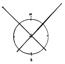
Fig. 3: Two additional orbits which could be added to those shown in Figs. 1 and 2. These orbits are inclined at  $\pm$  46.4°. Their eccentricity is 0.38.
