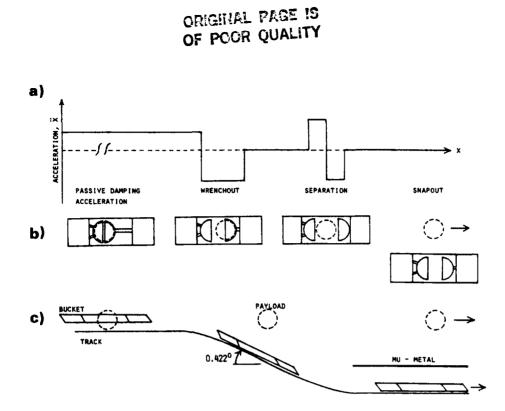
Figure 5. Separation and snapout. (a) Acceleration on bucket,  $\ddot{x}$ , as schematic function of along-track distance x. (b) Separation of payload from bucket; see text for discussion. (c) Detail of snapout; note mu-metal barrier.
