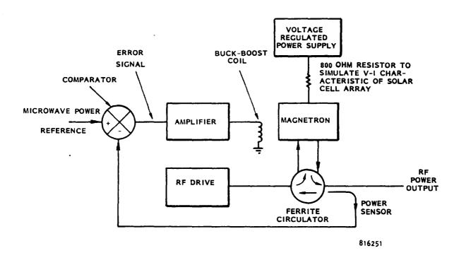
Figure 3. Test Arrangement for Evaluation of Amplitude Control.
