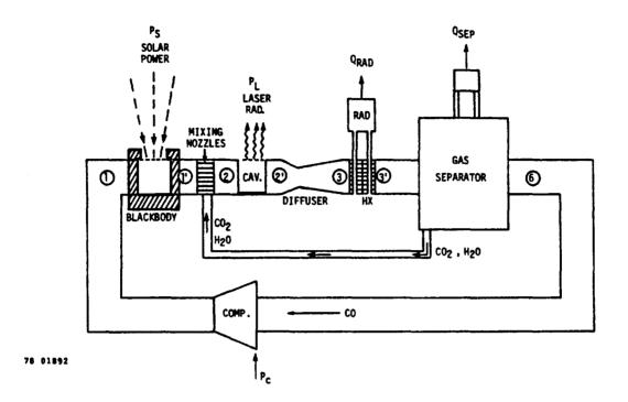
Figure 1. Indirect Optically Pumped  $CO/CO_2$  Mixing Laser
