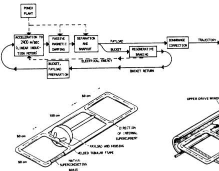
Figure 2. Mass-driver bucket. Frame is cut away to show superconducting braid. Note payload constraint/release system. (Modified from Chilton et. al., op. cit., p. 50)
