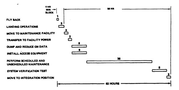
Figure 5- HLLV BOOSTER PROCESSING TIMELINES
