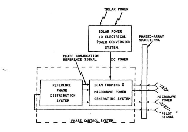
Figure 1. Solar Power Satellite (SPS) Transmission System (Phase Conjugation).
