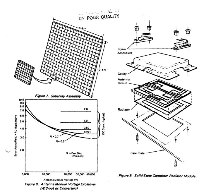
subarray. The main features of the combiner radiator module are illustrated in Figure 8. The modules would be integrated into any antenna panel of 8 modules. Each module radiates about 30 watts of linearly polarized RF power. This concept is a more direct substitution for klystrons and can be adapted to the SPS configurations shown in Figures 1 and 3.
