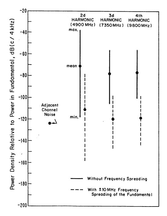
Figure 1. Estimates of interference levels in a 4 kHz bandwidth.
