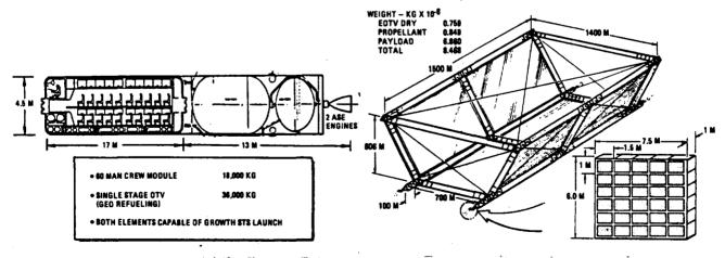
Figure 3. Personnel Orbital Transfer Vehicle
