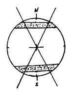
Fig. 1: Two near circular orbits inclined at ± 63.4°, could supply base load power to miniature rectennas between 40° and 60° latitude. These could provide for Europe's continuous power needs plus intermitent power to lower latitudes.
