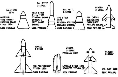
Figure 1- SPS LAUNCH VEHICLE CONCEPT EVOLUTION
