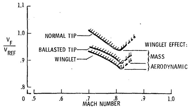
Fig. 10 Winglet effect on wing flutter speed.
