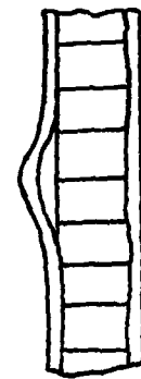
TENSILE BOND RUPTURE
