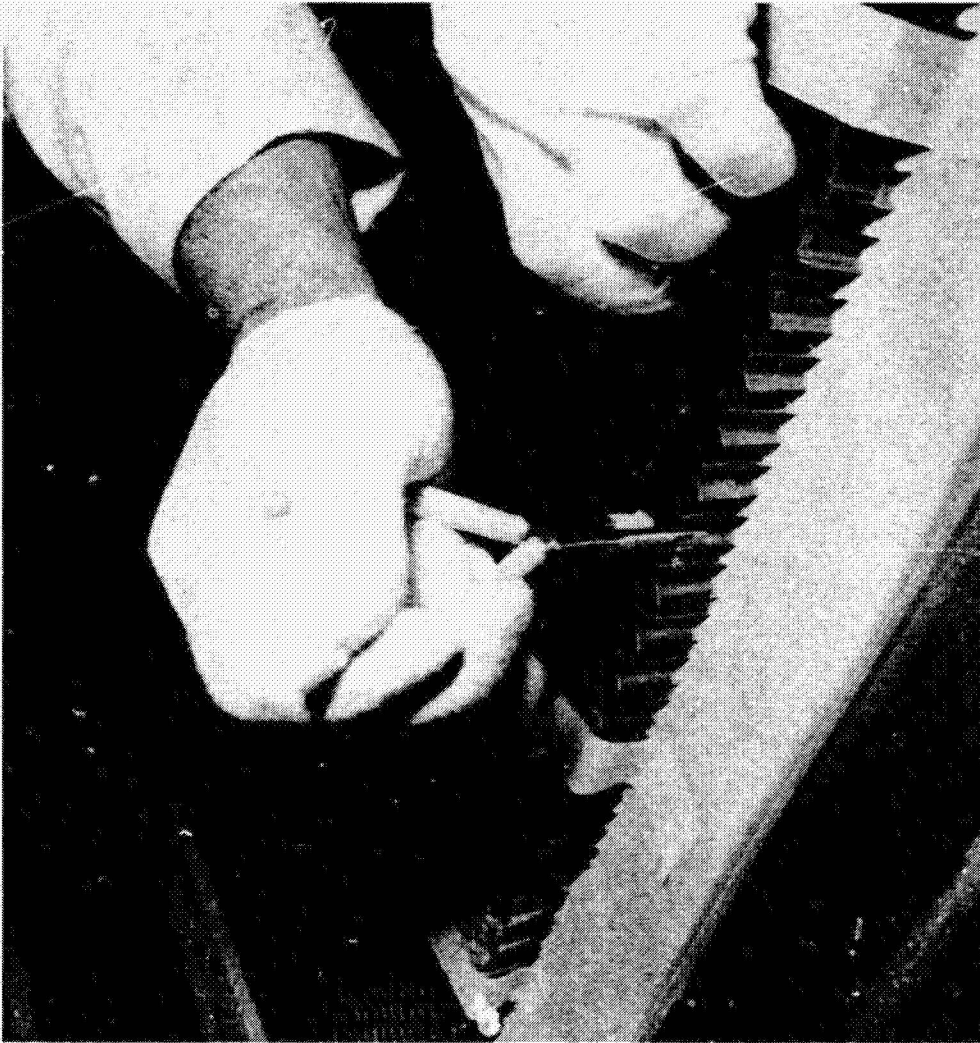
Figure 36.- Perforating honeycomb core at cell node points.
