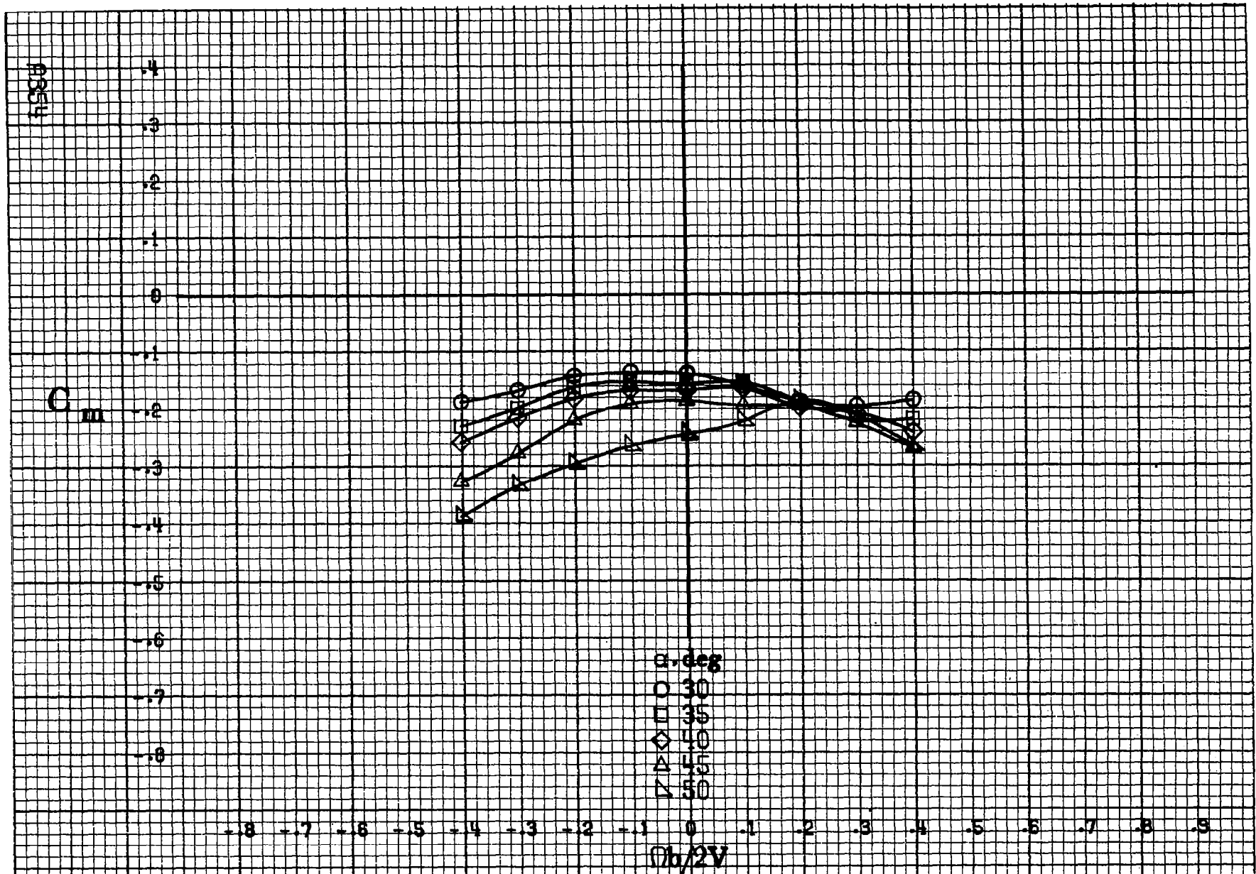
Figure A111.- Effect of rotation rate and angle of attack on pitching-moment coefficient for basic configuration. \delta_1 = 10^\circ , \delta_2 = -20.0^\circ , \delta_3 = -6^\circ , \delta_4 = 30^\circ , \delta = 10^\circ
