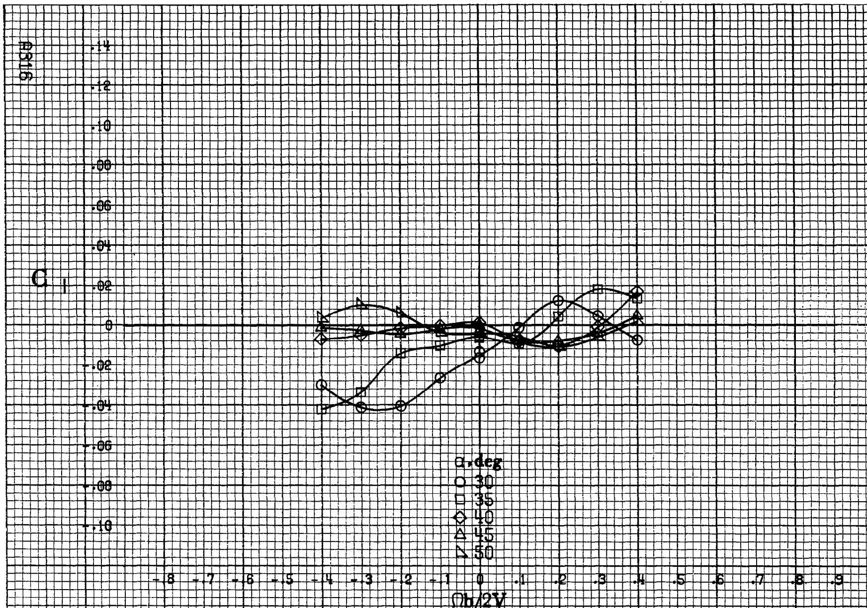
Figure A 92.- Effect of rotation rate and angle of attack on rolling-moment coefficient for basic configuration. \delta_a = 0^\circ , \delta_e = 20.0^\circ , \delta_a = 6^\circ , \delta_r = -15^\circ , \beta = 0^\circ .
