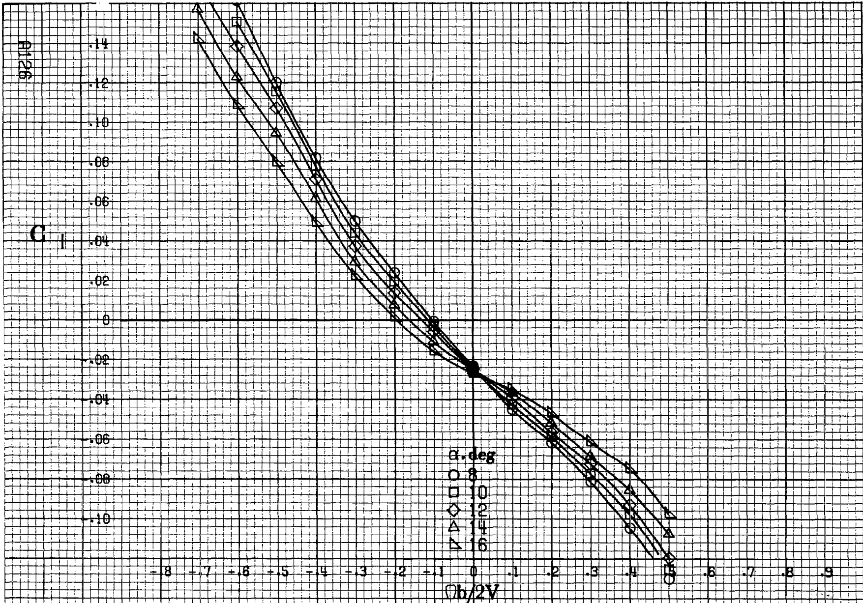
Figure A 32.-Effect of rotation rate and angle of attack on rolling-moment coefficient for basic configuration. \delta_e = 0^\circ , \delta_s = 0^\circ , \delta_d = 0^\circ , \delta_r = 0^\circ . \beta = 10^\circ .
