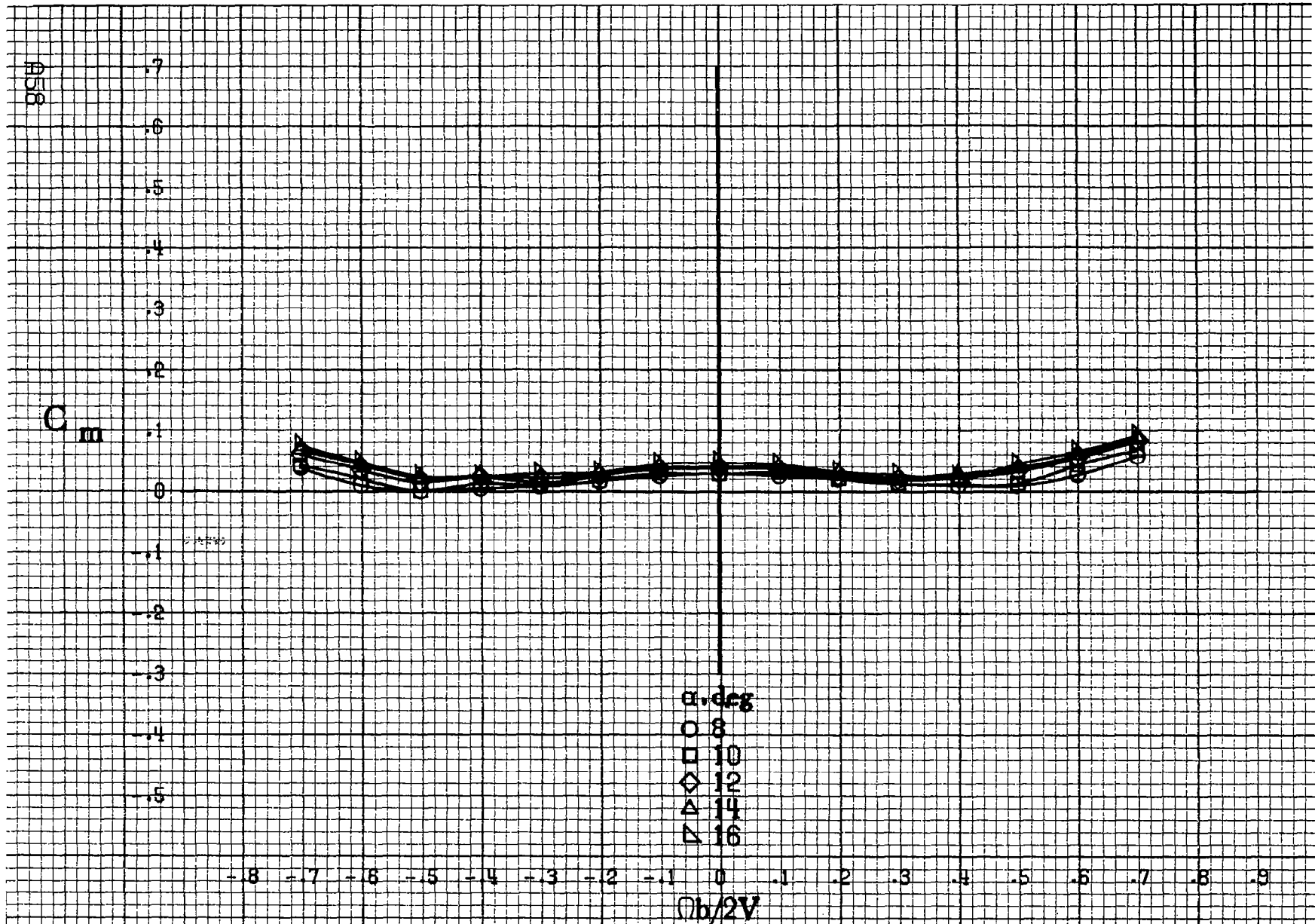
Figure A15.- Effect of rotation rate and angle of attack on pitching-moment coefficient for body wing vertical tail configuration. \delta_e = 0^\circ , \delta_a = 0^\circ , \delta_r = 0^\circ , \beta = 0^\circ .
