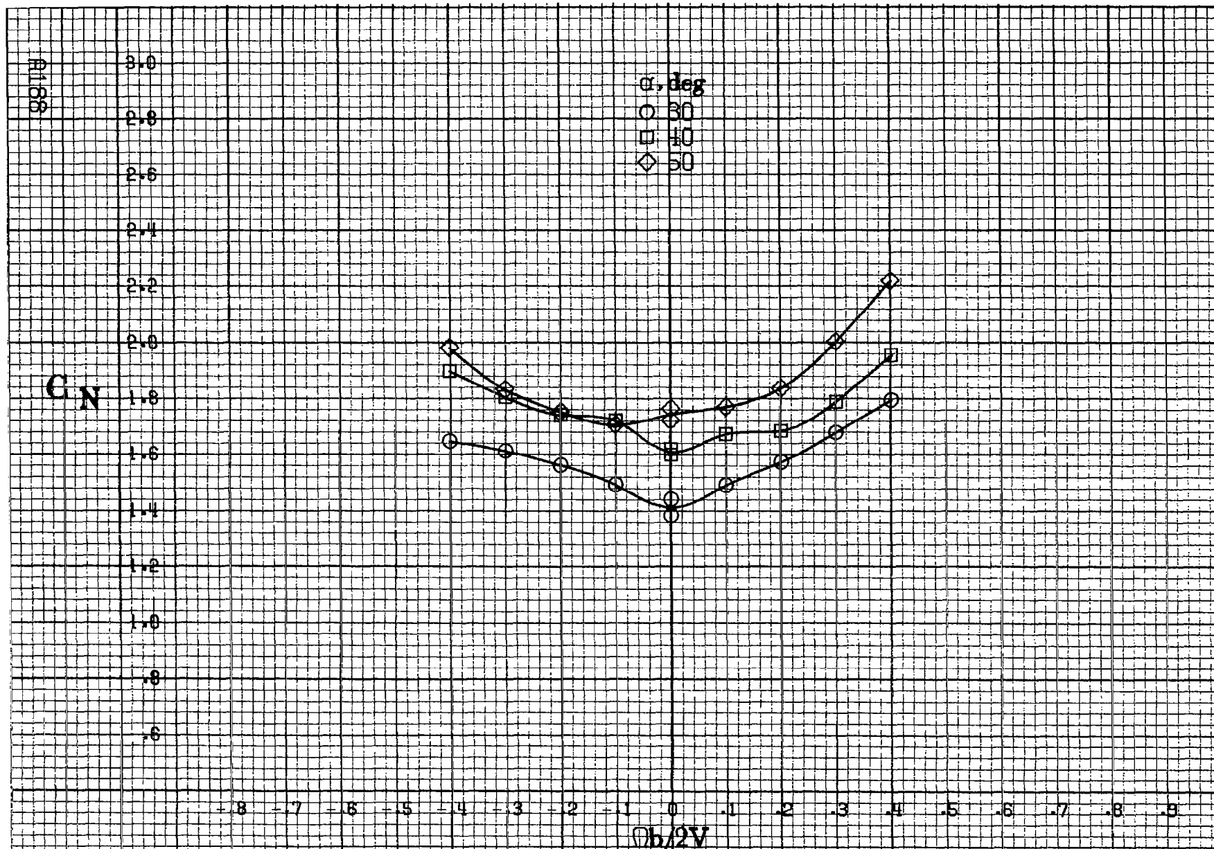
Figure A52.-Effect of rotation rate and angle of attack on normal-force coefficient for basic configuration. \delta_e = -25^\circ , \delta_a = 0^\circ , \delta_c = 0^\circ , \delta_r = 0^\circ . \beta = 10^\circ .
