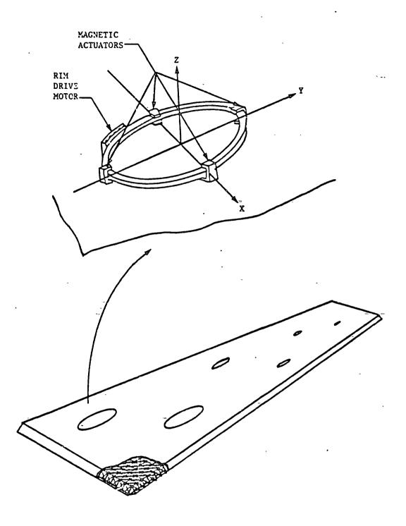
Figure 3. AMCD/LSS configuration.
