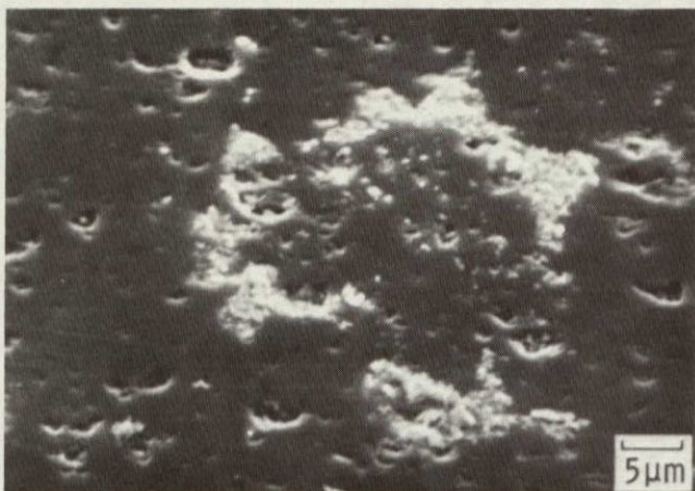
(a) SINTERED POLYCRYSTALLINE SILICON CARBIDE SURFACE; LOAD, 0.1N.
