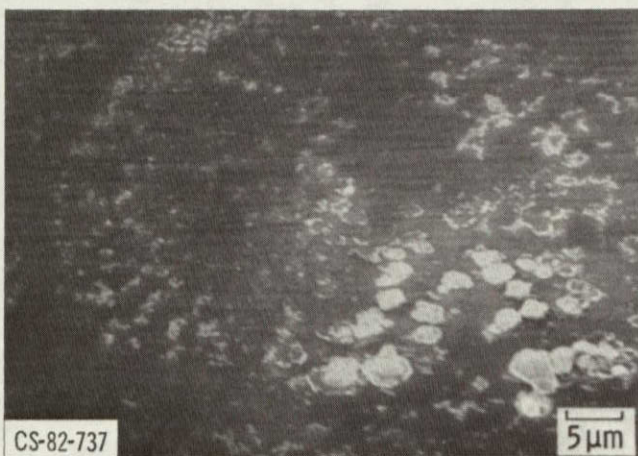
(b) SINGLE CRYSTAL SILICON CARBIDE {0001} SURFACE; SLIDING DIRECTION, \langle 10\bar{1}0 \rangle ; LOAD, 0.2N.
