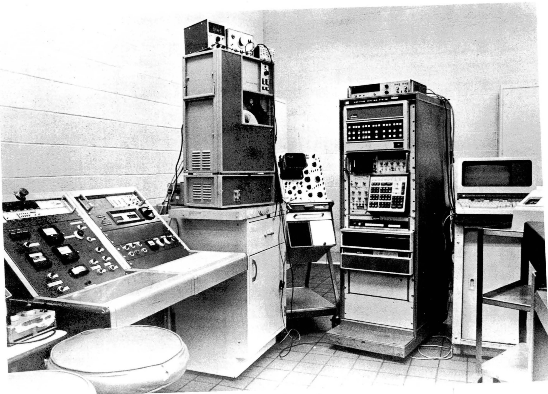
Control Console with Data Reduction Equipment
