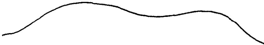
c) Final curve - ball has been rolled from below and above curve, with correction for offset of ball's radius
