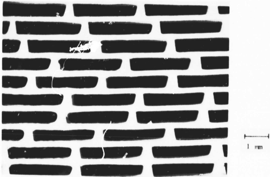
Figure 13. Enlarged Cross Section of Honeycomb
