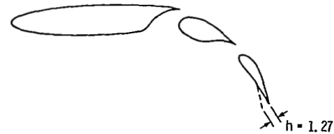
Configuration 5 with ramp trailing edge screen
