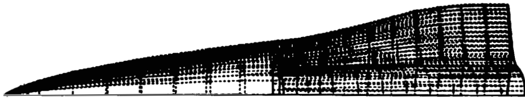
Figure 8.- Transition section smoothly fitted on to forebody.
