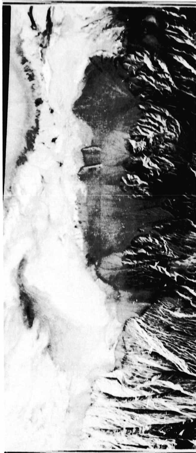
Figure 39. Thermal inertia image of the southern half of Death Valley produced from data obtained during the NP-3A flight on March 11, 1977.
