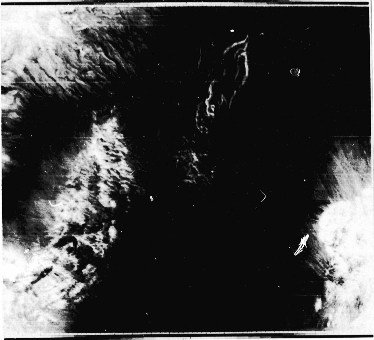
Figure 60. Thermal inertia image of Cuprite Mining District, Nevada from aircraft data. Image size is 8 x 12 km.
