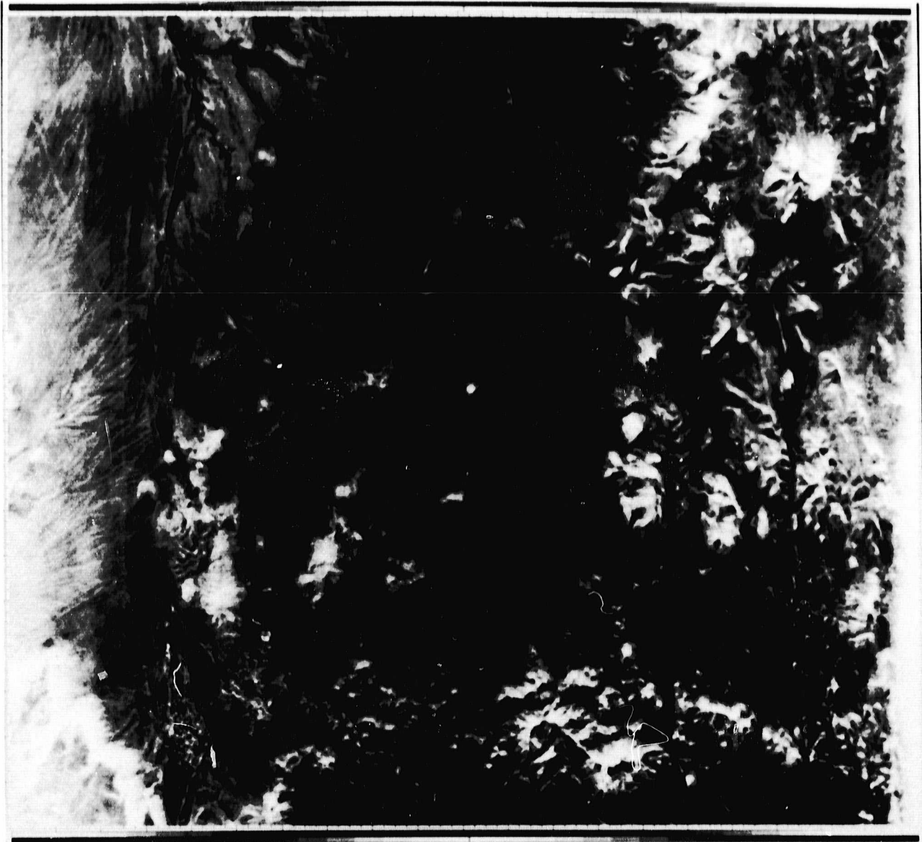
Figure 56. Thermal inertia image of Goldfield, Nevada from aircraft data. Image size is 15 x 15 km.
