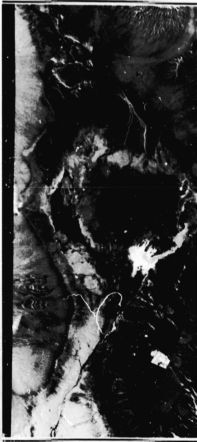
Figure 38. Thermal inertia image of the northern half of Death Valley produced from data obtained during the NP-3A flight on March 11, 1977.
