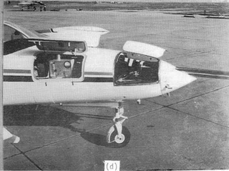
Figure 1.- (a) In situ aircraft; (b) nose probes; (c) instrumentation within main cargo area; and (d) forward compartment instrumentation.
