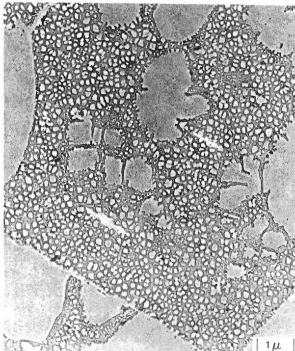
Figure 29 Micrographs of the Bore (Thick) Region of a Quarter Section of Disk 34D-1 Heat Treated at 1163^{\circ}\text{C} ( 2125^{\circ}\text{F} )/2 hrs Furnace Cool at 55^{\circ}\text{C} ( 100^{\circ}\text{F} ) Per Hour to 1121^{\circ}\text{C} ( 2050^{\circ}\text{F} )/0.5 hr/Salt Quench at 177^{\circ}\text{C} ( 350^{\circ}\text{F} )/AC + 649^{\circ}\text{C} ( 1200^{\circ}\text{F} )/2400 hrs/AC + 760^{\circ}\text{C} ( 1400^{\circ}\text{F} )/ 16 Hrs/AC Showing a Matrix Cooling Gamma Prime (Arrow) of Approximately 0.1\mu\text{m}
