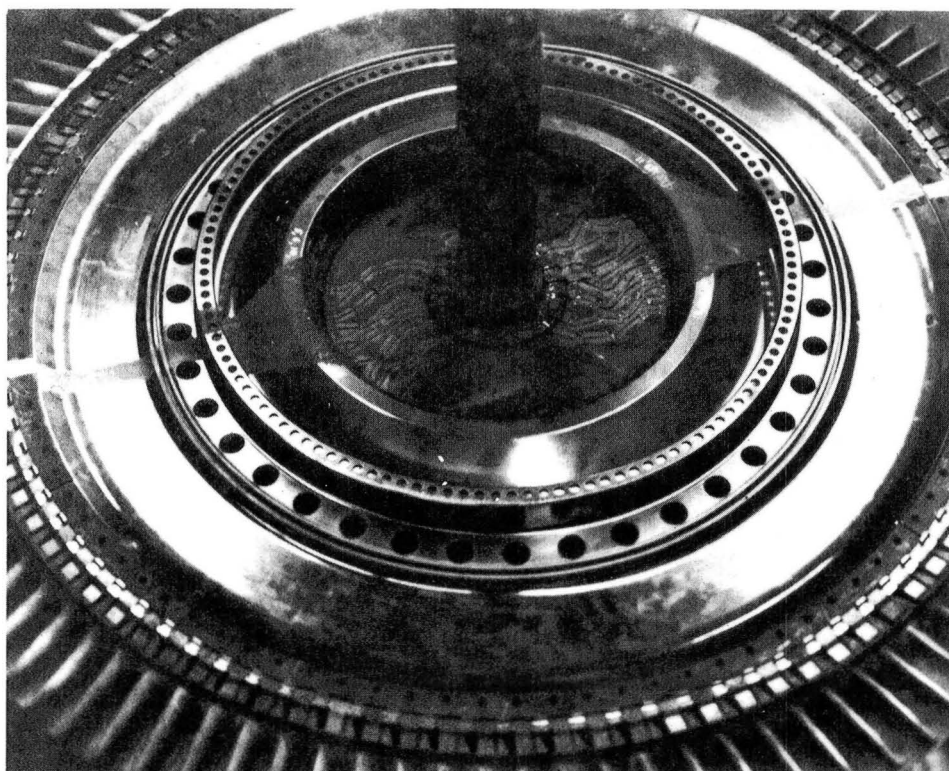
Figure 94 Location of Thermocouples Installed for Hot Spin Test
