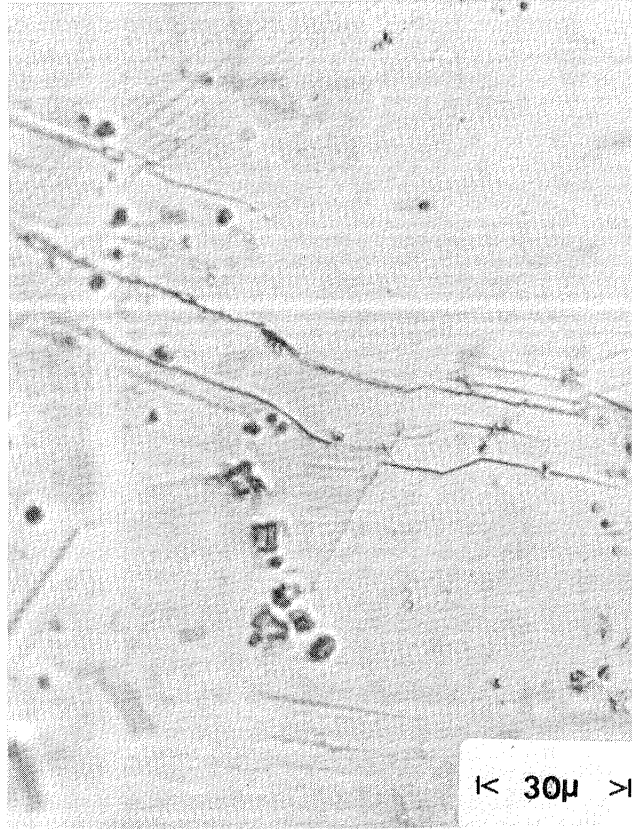
Figure 47 Coarse grained small \gamma specimen Ni 2 ( \Delta\epsilon_p = 0.15\% ). Slip band cracking was evident at 12000 cycles.
