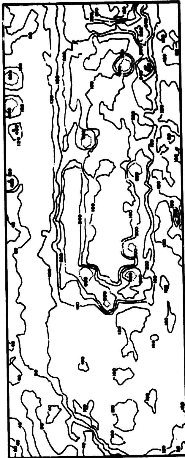
FIGURE 12 CONTOUR MAP OF SURFACE RETURN INTENSITY FROM RUNWAY AREA WITH DEPLOYED RETRO-REFLECTORS. DOTTED CONTOURS SURROUND REGIONS OF MAXIMUM RETURN INTENSITY.
