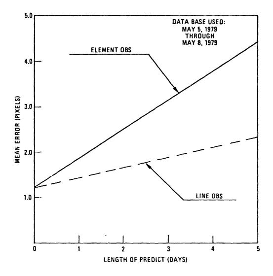
Figure 1. Line and pixel navigation prediction error for GOES VAS.
