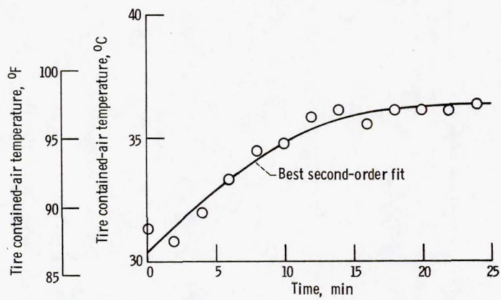
Figure 8. - Tire contained-air temperature as a function of time for constant-speed test. Speed, 56 km/hr (35 mph).
