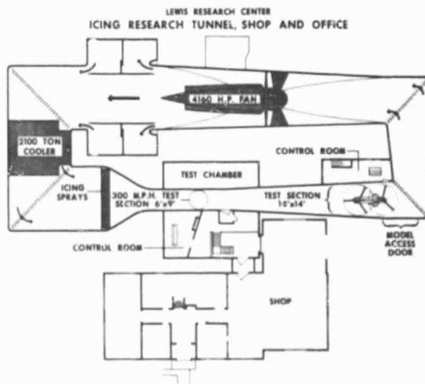
Figure 8 - Loop schematic of the Lewis Icing Research Tunnel.
