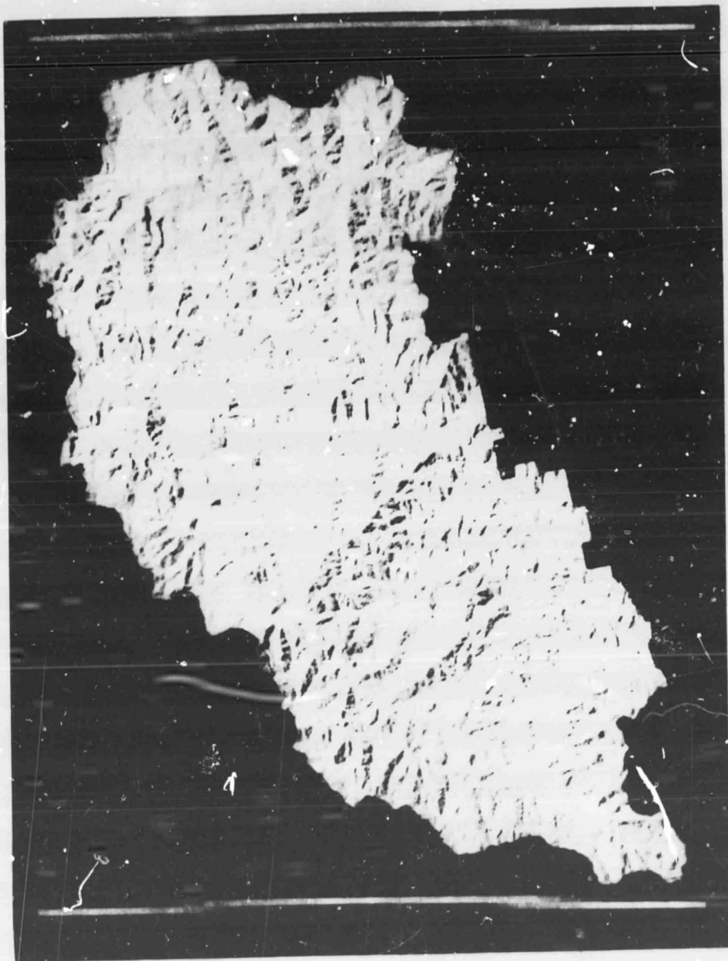
Figure 9. COSINE OF THE ZENITH ANGLE. This image displays the cosine of the angle between a normal to the slope and the sun at the time of the Landsat overpass. Bright areas correspond to slopes oriented directly toward the sun, and the darkest areas represent shadowed terrain. The image gives a strong visual impression of a landscape model illuminated from the southeast.
