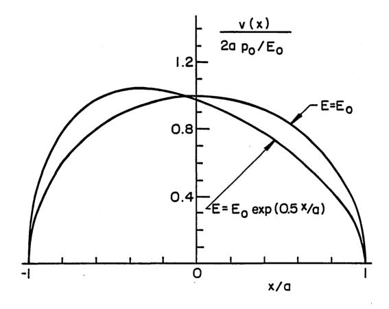
Fig. 3. Crack surface displacement v(x) in a nonhomogeneous and a homogeneous medium under uniform pressure  $p_0$  applied to the crack surfaces.  $(E(x) = E_0 \exp(0.5x/a)$  for the nonhomogeneous medium,  $E(x) = E_0$  for the homogeneous medium, v = 0.5,  $\beta a = 0.5$ , plane stress conditions).
