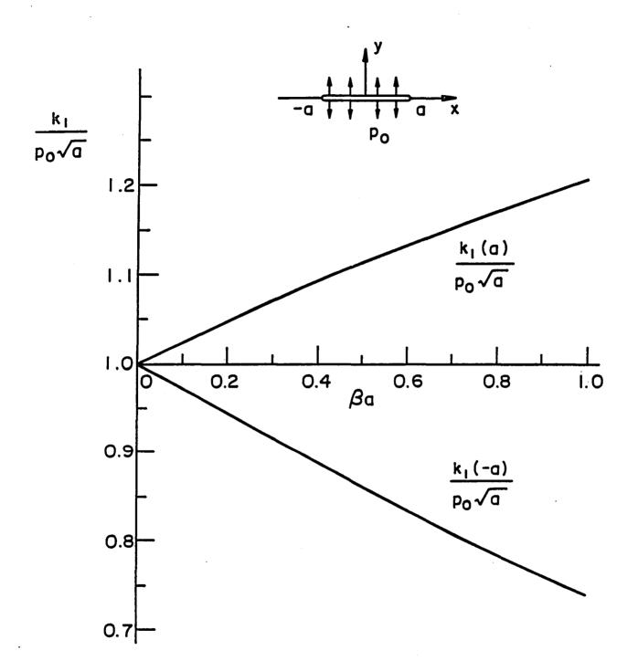
Fig. 2. Stress intensity factors in a nonhomogeneous medium having a uniformly pressurized crack ( $E(x) = E_0 e^{\beta X}$ , v = 0.3, plane stress conditions).
