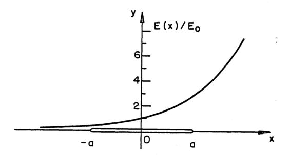
Fig. 1. The crack geometry in the nonhomogeneous medium and the variation of the Young's modulus  $E = E_0 e^{\beta X}$ .
