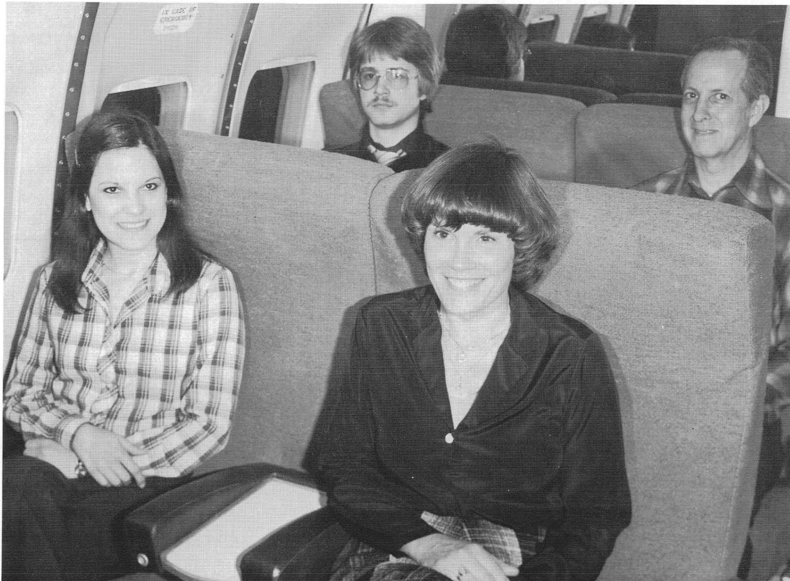
Figure 1.- Passenger ride quality apparatus at the Langley Research Center with front bulkhead removed.
