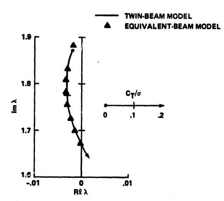
Fig. 23 Root locus plot of lead-lag mode of stiff-inplane, stiff-intorsion twinbeam model (zero inboard pitch); coupling structural stiffness terms of nonlinear origin suppressed in flutter analysis);  $\omega_v = 1.87\Omega$ ,  $\omega_w = 1.15\Omega$ ,  $\omega_\phi = 5.38\Omega$ ,  $\gamma = 5.0$ ,  $\beta_p = 0.05$  rad.
