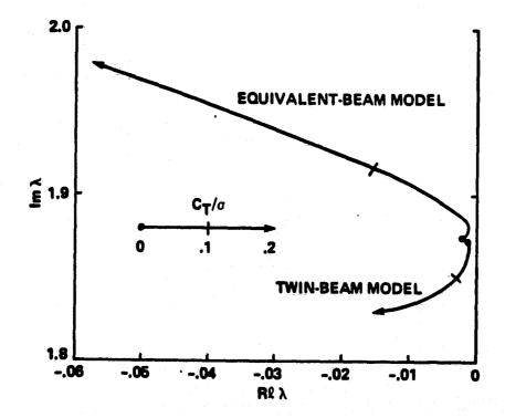
Fig. 26 Root locus plot of lead-lag mode of stiff-inplane, stiff-in-torsion twinbeam model (same pitch for inboard and outboard);  $\omega_v = 1.87\Omega$ ,  $\omega_w = 1.15\Omega$ ,  $\omega_\phi = 5.38\Omega$ ,  $\gamma = 5.0$ ,  $\beta_p = 0.05 \, rad$ .
