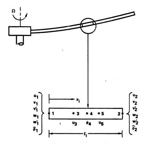
Fig. 15 Refined finite element for multiple-load-path blades.
