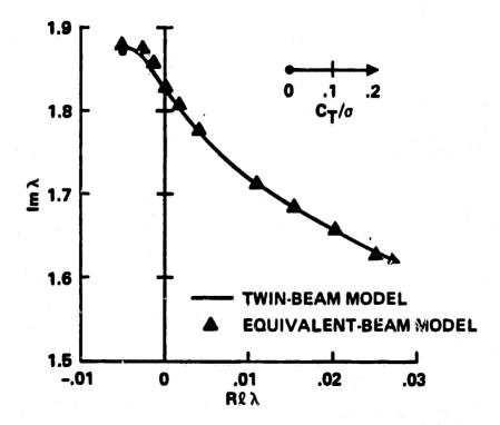
Fig. 19 Root locus plot of lead-lag mode of stiff-inplane, soft-in-torsion twinbeam model (zero inboard pitch; coupling structural stiffness terms of nonlinear origin suppressed in flutter analysis);  $\omega_v = 1.87\Omega$ ,  $\omega_w = 1.15\Omega$ ,  $\omega_{\phi} = 2.91\Omega$ ,  $\gamma = 5.0$ ,  $\beta_p = 2.05 \, rad$ .
