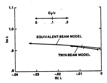
Fig. 20 Root locus plot of lead-lag mode of soft-inplane, soft-intorsion twinbeam model (zero inboard pitch);  $\omega_v = 0.90\Omega$ ,  $\omega_w = 1.15\Omega$ ,  $\omega_\phi = 2.91\Omega$ ,  $\gamma = 5.0$ ,  $\beta_p = 0.05 \, rad$ .
