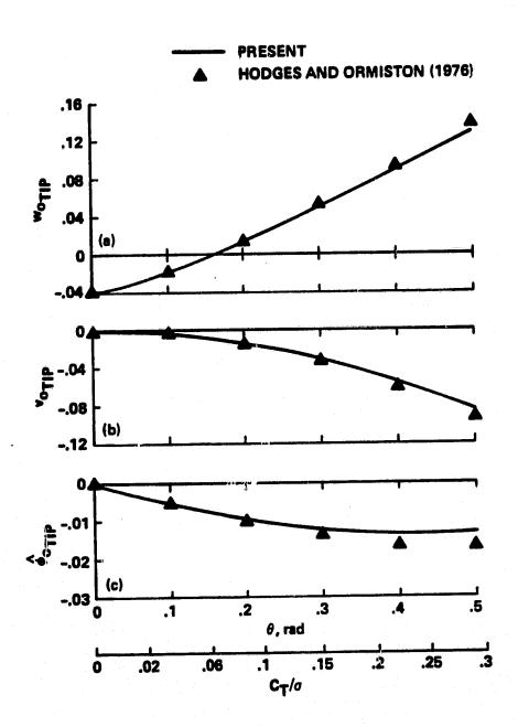
Fig. 8 (a) Flap bending (b) lead-lag bending (c) torsion. Steady tip deflections of a soft-inplane hingeless rotor blade;  $\omega_v = 0.7\Omega$ ,  $\omega_w = 1.15\Omega$ ,  $\omega_\phi = 5.0\Omega$ ,  $\gamma = 5.0$ ,  $\beta_p = 0.05$  rad.
