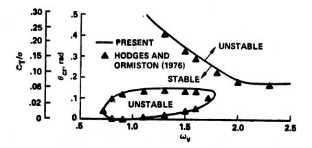
Fig. 10 Stability boundaries for a hingeless rotor blade;  $\omega_w = 1.15\Omega$ ,  $\omega_{\phi} = 2.5\Omega$ ,  $\gamma = 5.0$ ,  $\beta_p = 0.05 \, rad$ .
