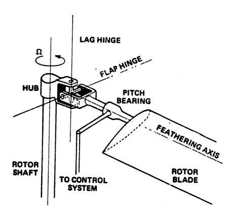
Fig. 1 Schematic of an articulated rotor hub and root.
