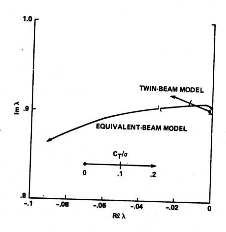
Fig. 25 Root locus plot of lead-lag mode of soft-inplane, soft-in-torsion twinbeam model (same pitch for inboard and outboard);  $\omega_v = 0.90\Omega$ ,  $\omega_w = 1.15\Omega$ ,  $\omega_{\phi} = 2.91\Omega$ ,  $\gamma = 5.0$ ,  $\beta_p = 0.05 \, rad$ .
