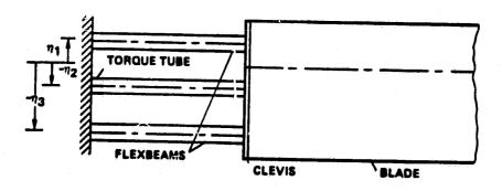
Fig. 14 Analytical model of a bearingless blade.
