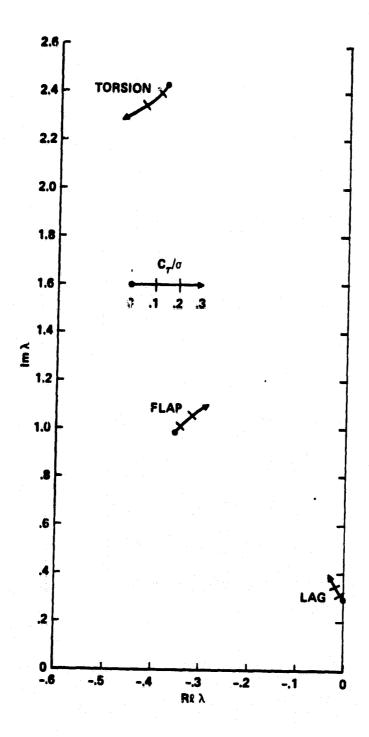
Fig. 13 Root locus plot for an articulated rotor blade; hinge offset=0.06R,  $\omega_{\phi} = 2.5\Omega$ ,  $\gamma = 5.0$ ,  $\beta_{p} = 0.05 \, rad$ .
