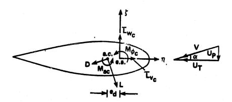
Fig. 5 Deformed-blade-section aerodnamics
