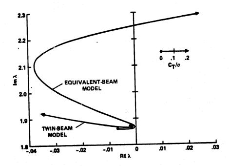
Fig. 24 Root locus plot of lead-lag mode of stiff-inplane, soft-in-torsion twinbeam model (same pitch for inboard and outboard);  $\omega_v = 1.87\Omega$ ,  $\omega_w = 1.15\Omega$ ,  $\omega_{\phi} = 2.91\Omega$ ,  $\gamma = 5.0$ ,  $\beta_p = 0.05 \, rad$ .
