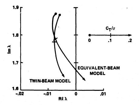
Fig. 22 Root locus plot of lead-lag mode of stiff-inplane, stiff-intorsion twinbeam model (zero inboard pitch);  $\omega_v = 1.87\Omega$ ,  $\omega_w = 1.15\Omega$ ,  $\omega_\phi = 5.38\Omega$ ,  $\gamma = 5.0$ ,  $\beta_p = 0.05 \, rad$ .
