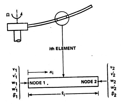
Fig. 6 A finite element showing nodal degrees of freedom
