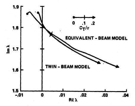
Fig. 18 Root locus plot of lead-lag mode of stiff-inplane, soft-intersion twinbeam model (zero inboard pitch);  $\omega_v = 1.87\Omega$ ,  $\omega_w = 1.15\Omega$ ,  $\omega_\phi = 2.91\Omega$ ,  $\gamma = 5.0$ ,  $\beta_p = 0.05 \, rad$ .
