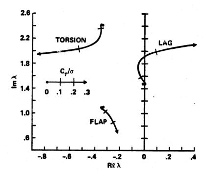
Fig. 9 Root locus plot for a hingeless rotor blade;  $\omega_v = 1.5\Omega$ ,  $\omega_w = 1.15\Omega$ ,  $\omega_\phi = 2.5\Omega$ ,  $\gamma = 5.0$ ,  $\beta_p = 0.05 \, rad$ .
