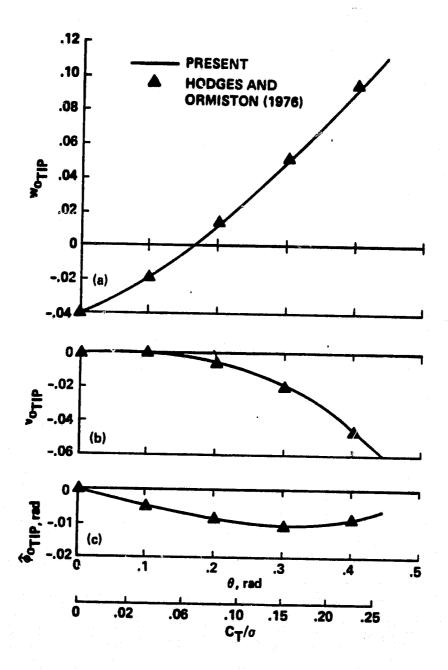
Fig. 7 (a) Flap bending (b) lead-lag bending (c) torsion. Steady tip deflections of a stiff-inplane hingeless rotor blade;  $\omega_v = 1.5\Omega$ ,  $\omega_w = 1.15\Omega$ ,  $\omega_{\phi} = 5.0\Omega$ ,  $\gamma = 5.0$ ,  $\beta_p = 0.05 \, rad$ .
