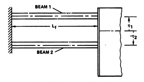
Fig. 17 Twinbeam multiple-load-path blade model.
