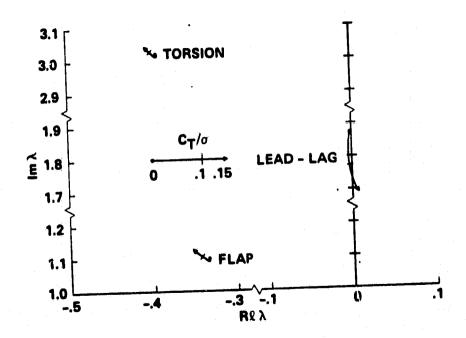
Fig. 27 Root locus plot of a bearingless blade with two identical flexbeams and a torque tube;  $\omega_v = 1.87\Omega$ ,  $\omega_w = 1.15\Omega$ ,  $\omega_{\phi} = 3.10\Omega$ ,  $\gamma = 5.0$ ,  $\beta_p = 0.05 \, rad$ .
