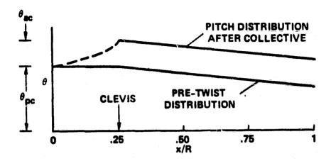
Fig. 16 Pitch distribution of a bearingless rotor blade.
