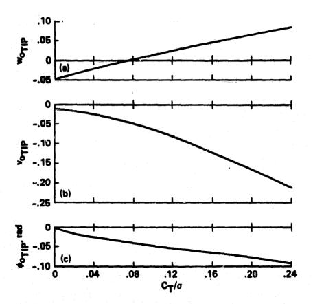
Fig. 12 a) Flap bending, b) lead-lag bending c) torsion. Steady tip deflections of an articulated rotor blade; hinge offset=0.06R,  $\omega_{\phi} = 2.5\Omega$ ,  $\gamma = 5.0$ ,  $\beta_{p} = 0.05 \, rad$ .
