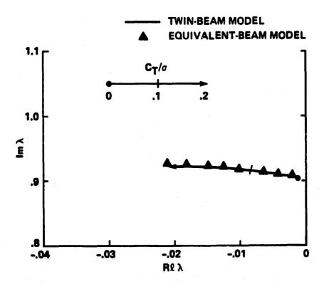
Fig. 21 Root locus plot of lead-lag mode of soft-inplane, soft-in-torsion twinbeam model (zero inboard pitch; coupling structural stiffness terms of nonlinear origin suppressed in flutter analysis);  $\omega_v = 0.90\Omega$ ,  $\omega_w = 1.15\Omega$ ,  $\omega_{\phi} = 2.91\Omega$ ,  $\gamma = 5.0$ ,  $\beta_p = 0.05 \, rad$ .
