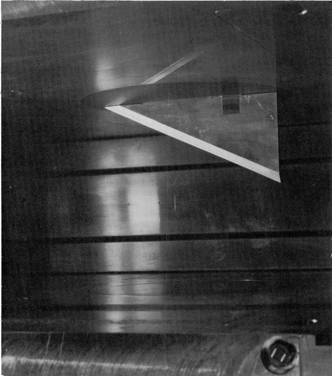
Figure 4.- Photograph of delta-wing buffet model mounted in the 0.3-Meter Transonic Cryogenic Tunnel with slotted floor in background.
