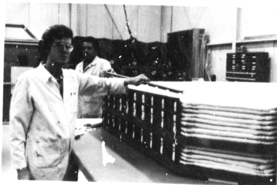
Figure VI-2. Assembly of two layers of radiators between, and on top of, two multiwire proportional chambers.
