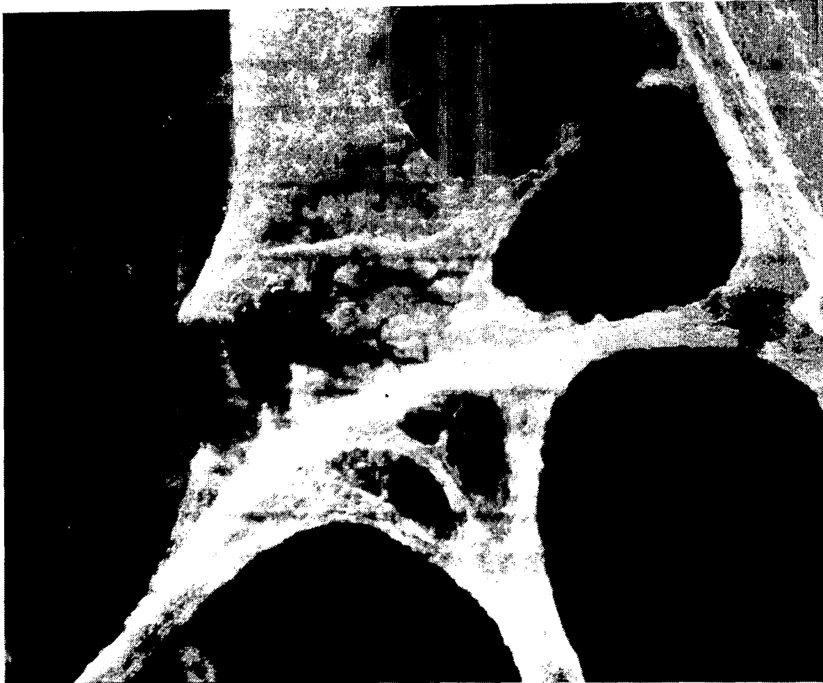
Figure 4-5. SEM of PCTFE fibers produced by In Situ Fiberization. Magnification \approx 1200\times .
