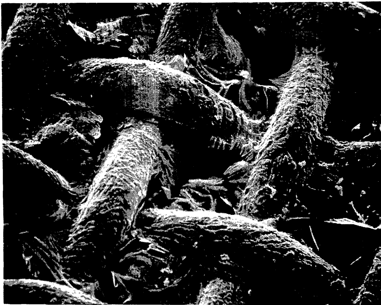
Figure 4-7. SEM of precipitate on a metal screen agitated in a poly p-phenylene terephthalamide/ \text{H}_2\text{SO}_4 solution. Magnification \approx 60\times .
