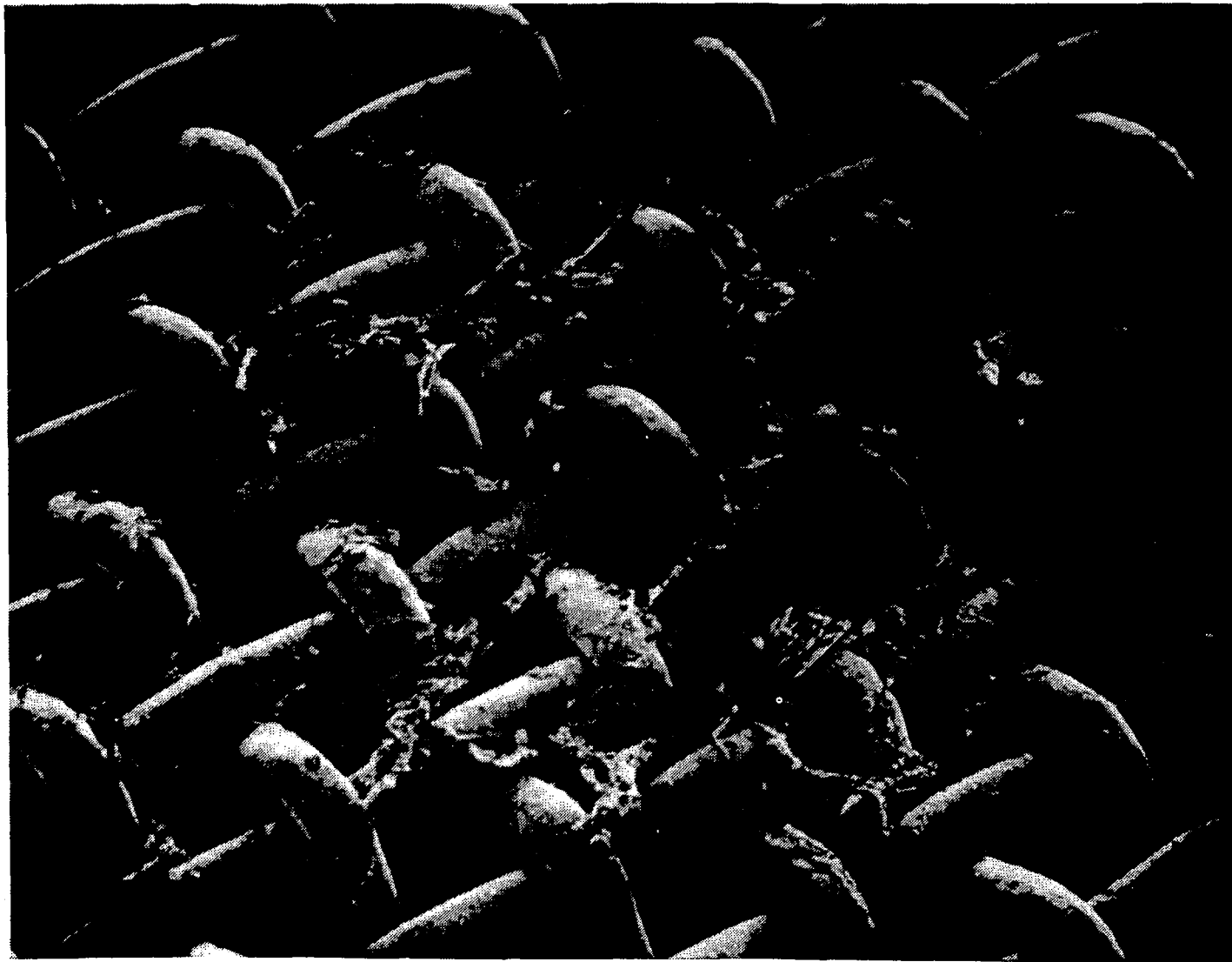
Figure 4-1. SEM of polyamic acid fibers formed on a brass screen agitated in a refluxing DMA solution. Magnification \approx 25X .
