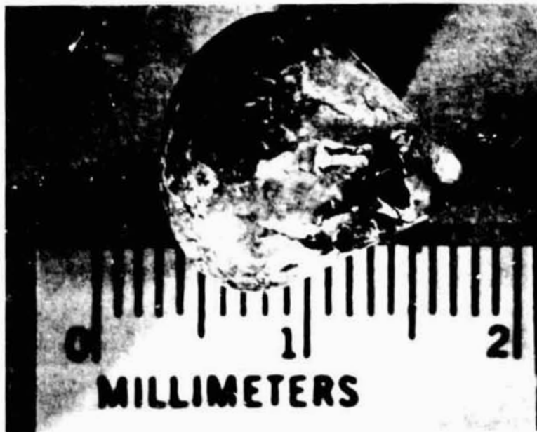
Figure 1. The appearance of a typical melt of Sm-Co alloy by R.F. Levitation.
