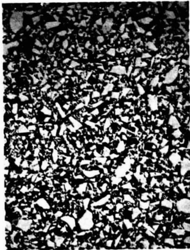
Figure 7. Photomicrograph of the SmCo 5 powder prepared by attritor ball milling in the comminution chamber.
